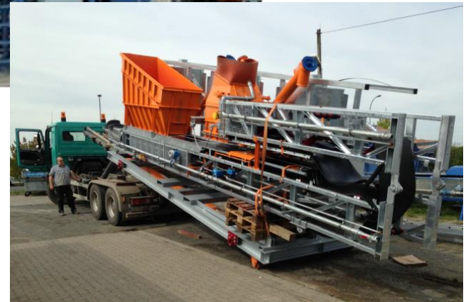
mobile construction site production in a compact unit for small-capacity building sites (eg 30–60 m 3 /h) (depending on the soil type)
