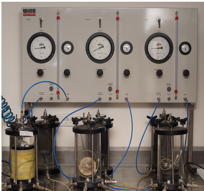
Triaxial cell for determining the k_f value
