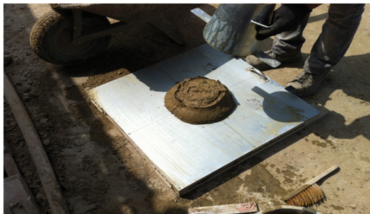
Determination of the diameter of flow for the purpose of cubature determination
